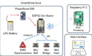
*Figure 2: Device Structure and Data Pipeline*
